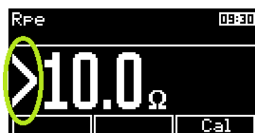
Figure 43: Measured value is out of range (max)
