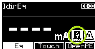
Figure 36: Warning concerning a DUT isolated placing
