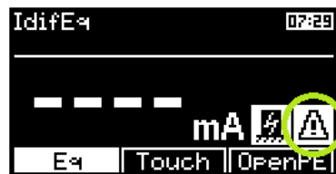
Figure 35: Warning concerning of a point of danger
