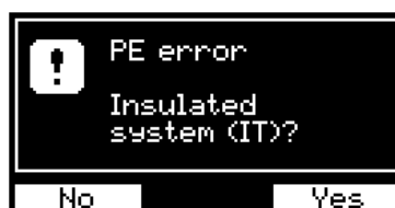
Figure 23: Warning message: PE error (IT systems)
