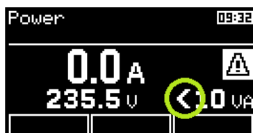
Figure 44: Measured value is out of range (min)
