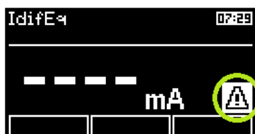
Figure 17: Warning concerning of a point of danger
