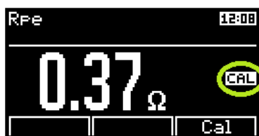
Figure 28: Incorrect compensation for the test leads
