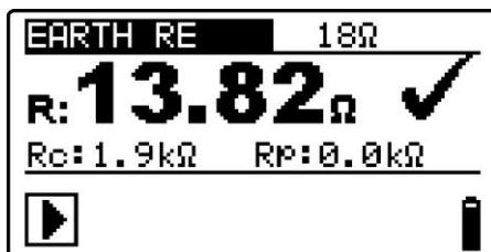
Figure 5.35: Example of earth resistance measurement result
