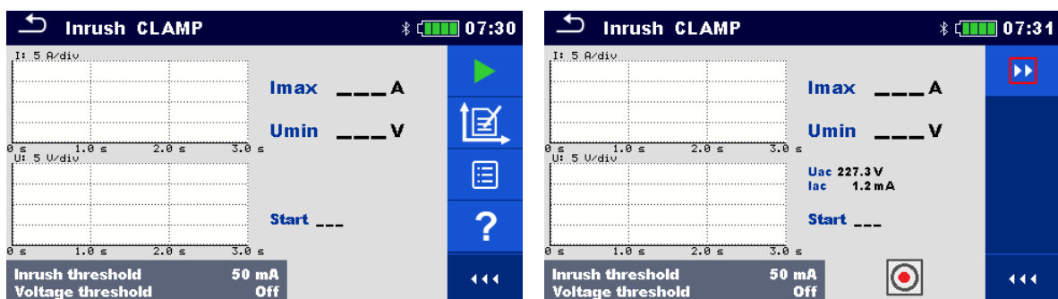
Figure 7.157: Inrush CLAMP menu – setup on the left, waiting for trigger on the right
