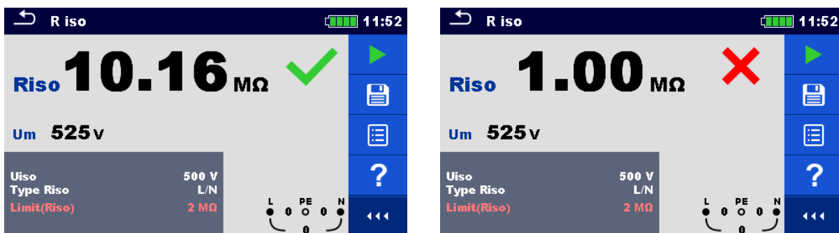
Figure 7.9: Examples of Insulation resistance measurement result
