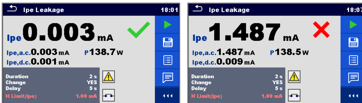
Figure 6.46: Examples of I pe Leakage measurement results
