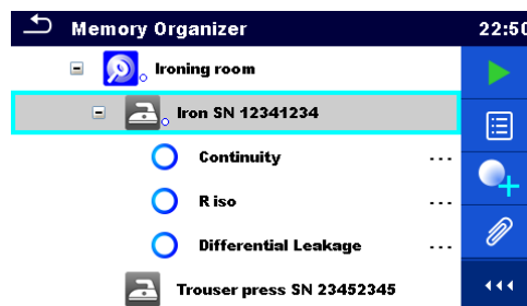
Figure 5.3: Example of status - No measurement result(s)
