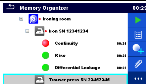
Figure 5.5: Status - Measurements completed with fail result(s)
