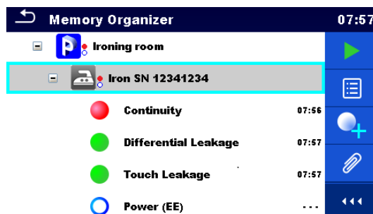
Figure 5.4: Example of status - Measurements not completed with fail result(s)
